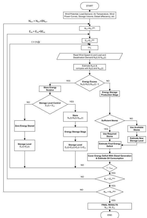
Figure 5. The developed simulation algorithm
