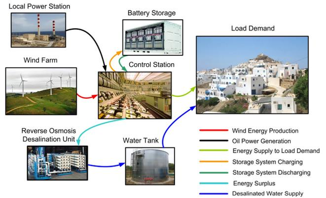
Figure 4. The proposed wind-based energy and water supply configuration
