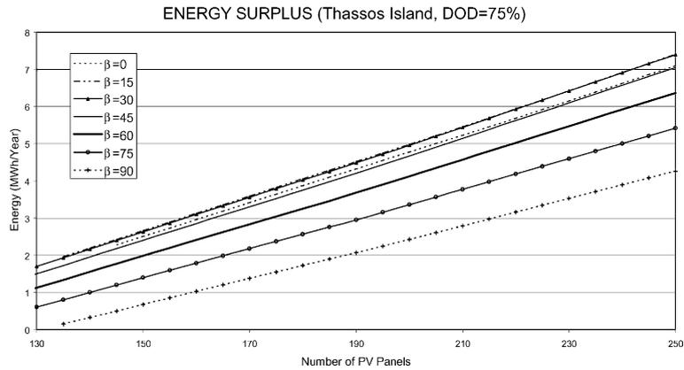
Fig. 15. Energy surplus of an autonomous PVS in Thassos island.
