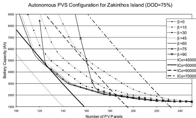
Fig. 12. Optimum autonomus PVS configuration for Zakynthos island.
