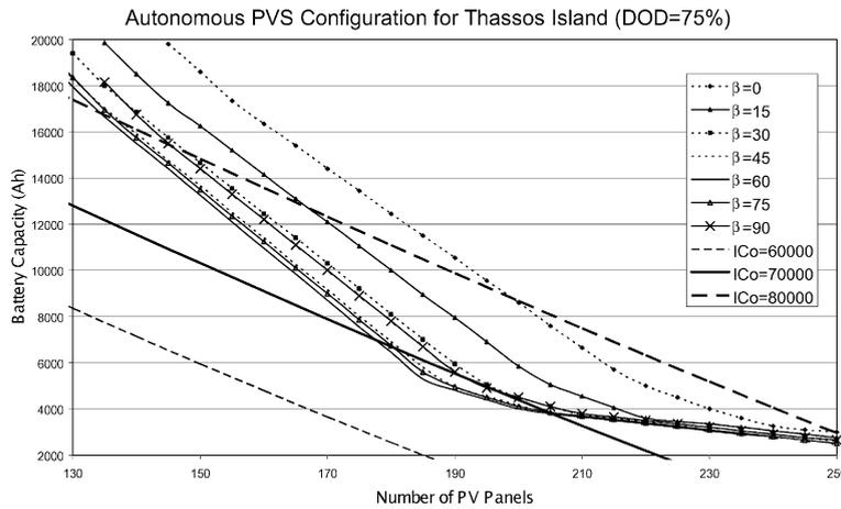
Fig. 14. Optimum autonomous PVS configuration for Thassos island.
