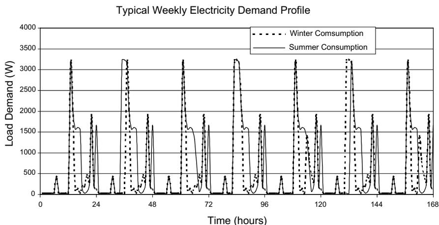
Fig. 4. Typical electricity demand profile of the remote consumer analyzed.
