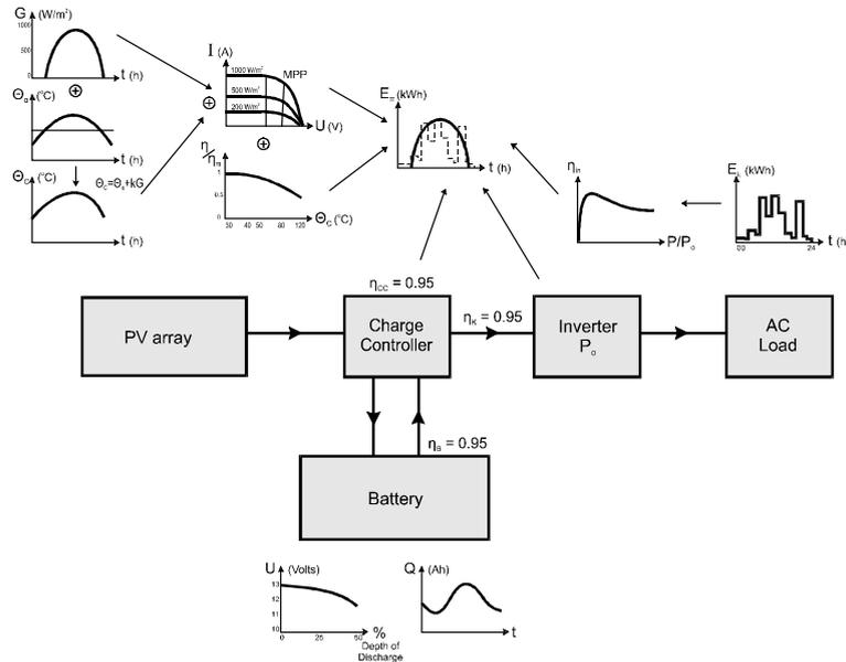
Fig. 3. Proposed autonomous PVS configuration for remote consumers.
