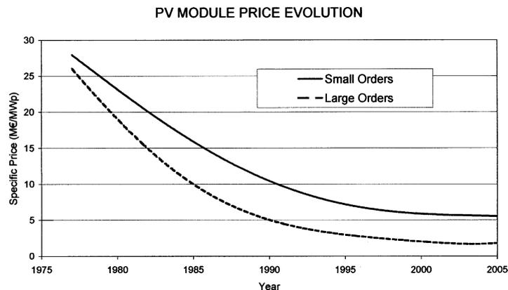
Fig. 1. Photovoltaic modules price evolution (estimation after 2002).
