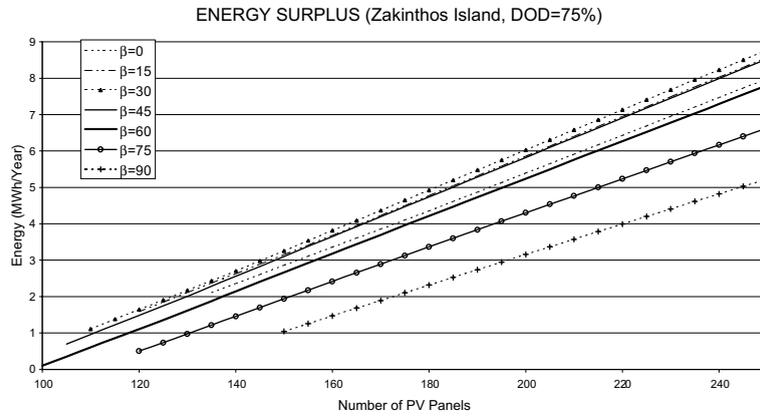
Fig. 13. Energy surplus of an autonomous PVS in Zakinthos island.
