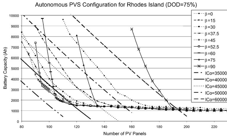
Fig. 8. Optimum autonomous PVS configuration for Rhodes island.
