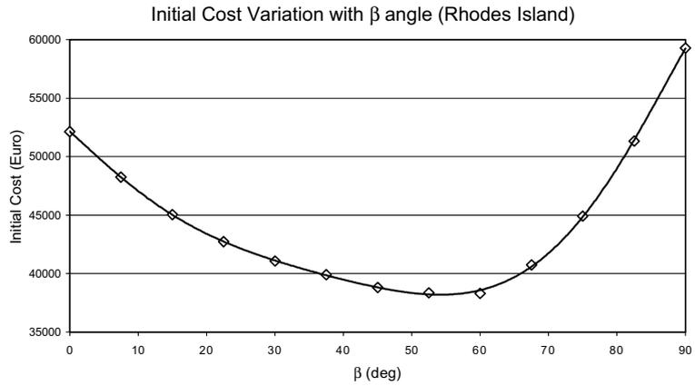
Fig. 9. Influence of panel tilt angle on first installation cost of an autonomous PVS.
