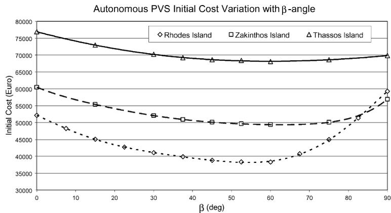
Fig. 16. Initial cost variation with panel tilt angle for typical Greek island PVSs.
