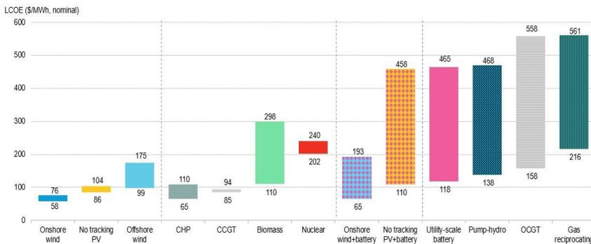
Figure 1 Levelized cost of electricity (LCOE) of major power generation technologies in Europe. (WindEurope 2019)
