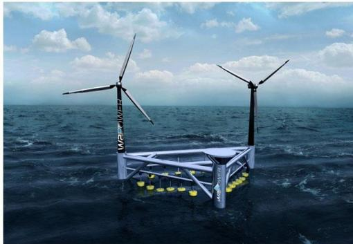
Figure 7 Example of Hybrid Wind Wave System (W2Power by Pelagic Power)
