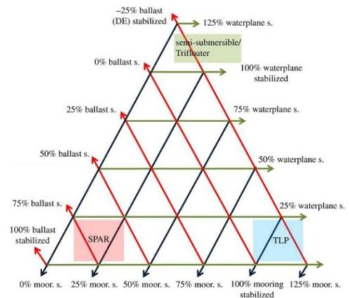
Figure 6 Stability triangle for floating structures
