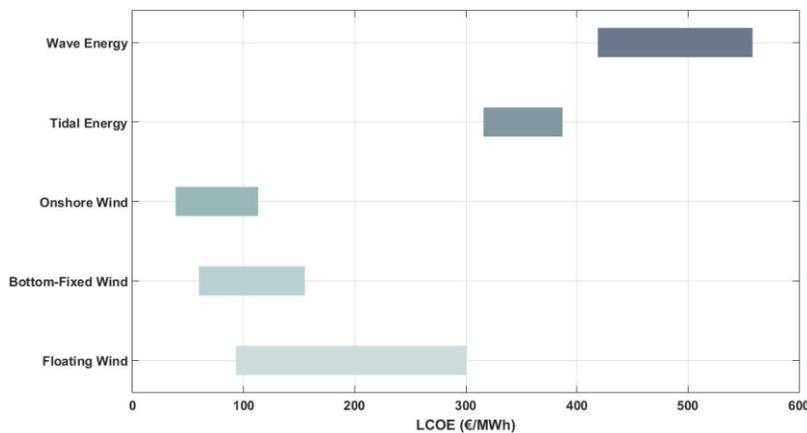
Figure 2 LCOE comparison between marine renewable energy generation technologies. LCOE values are taken from various sources from 2013 to 2019
