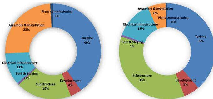
Figure 4 CAPEX breakdown; left: BOW; right: FOW
